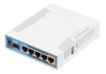
A dual concurrent 2.4 GHz / 5 GHz high power AP with five Gigabit Ethernet ports, SFP and PoE support.
